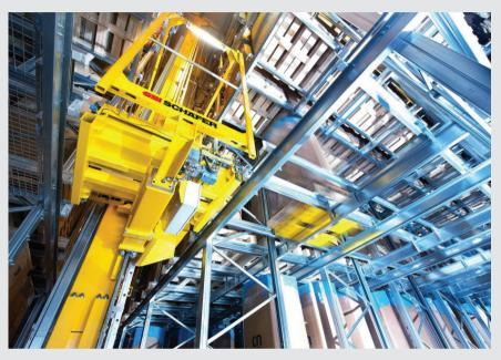
The Orbiter  $^{\text{TM}}$  can also be used in combination with automated storage and retrieval systems in deep-freeze environments.
